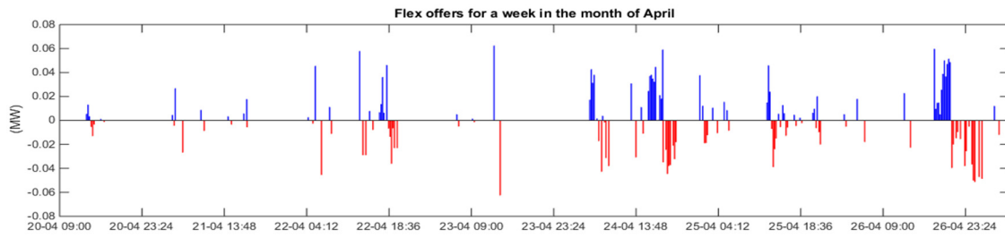
Figure 10 Flexible demand that has to be shifted to avoid voltage issues (blue) and shifted flexible demand to the next possible time slot to avoid grid issues (red).
