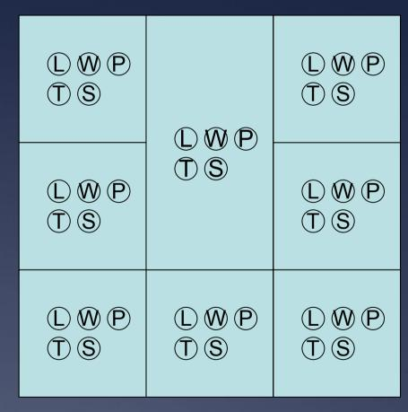
L=Lamp, W=heater, P=PIR, S=lux-sensor, T=temp-sensor
