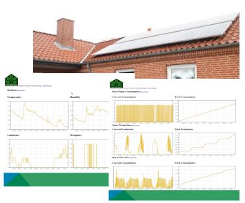
In the first demonstration, the project partners set up a real-life scenario (a private home in Aalborg) where different applications and devices (home gateway, solar panel, heat pump and in-house sensors) were integrated, exchanging data through the common interoperability middleware, hosted in a private cloud. A web application was able to collect data from the middleware database and provide information on sensor data as well as production and consumption graphs.
