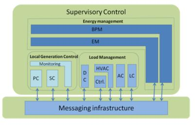
Figure 31 - Internal structure of Supervisory Control
