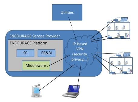
Figure 22 – ENCOURAGE IP-based connection
