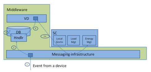
Figure 25 – Internal data conversion
