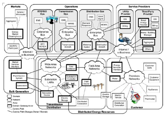
Figure 3 – Conceptual model for Smart Grid ICT [11]
